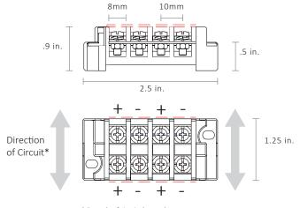
\* Example of circuit shown above, current on output side will match current of input side.
